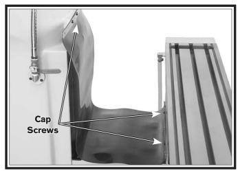
Figure 11. Rear way cover installed.
